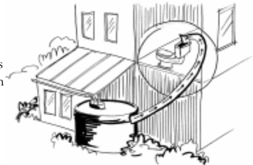
Water from the catchment system at the Reddick property will be used to flush toilets for the offices and apartments. Annual flushing will use about 53,000 gallons of rainwater from the roofs reducing the water collected from Eastsound Water Users Association's wells and reservoir
